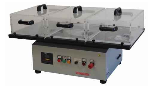
USED TO DETERMINE THE POTENTIAL FOR DISINTEGRATION OF TISSUE PAPERS IN WATER
